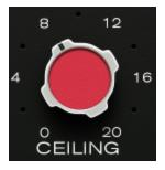
Increases the threshold and compensates the makeup level to keep a constant output level. The dynamics can be changed on the fly without changing the in / out settings.
